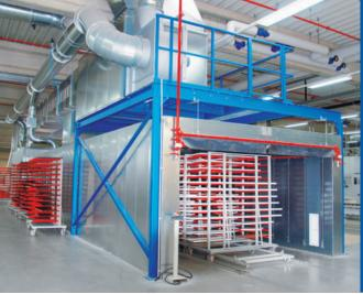
:: The energy consumption of a surface coating plant is substantially determined by the right choice of dryer. That applies equally to adhesive water dryers, powder enamelling furnaces or paint dryers. If one regards the total costs of a
